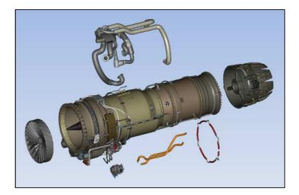
View a part/assembly in context view where the specific part/assembly is highlighted. For example, there are 4 major assemblies in a jet engine (fan, compressor, combustion & turbine). The compressor can be highlighted for user to understand its position and relation with respect to the whole engine.
